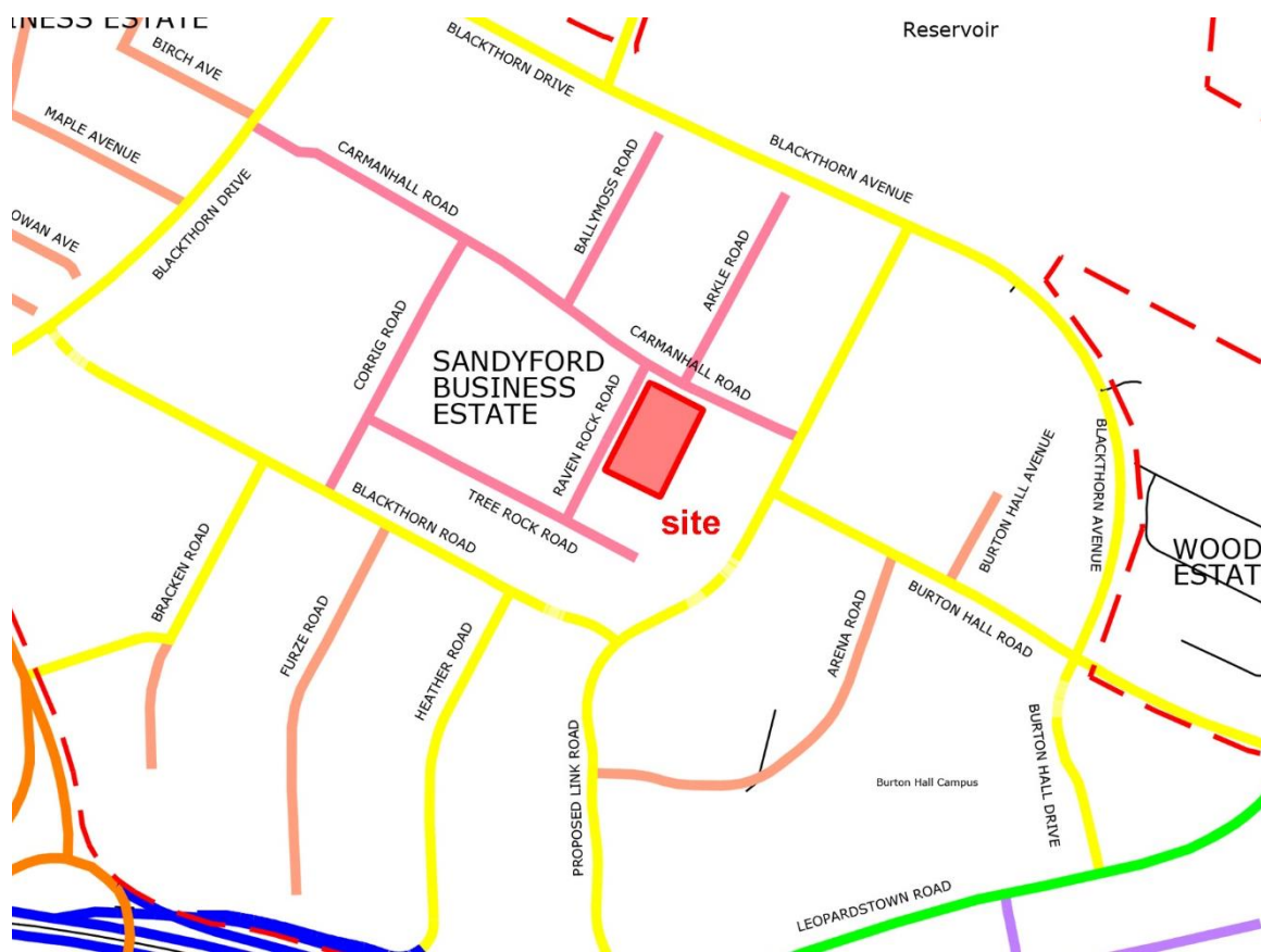
Figure 5 Sandyford Business Estate Road Hierarchy (SUFP Drg No 7) (Level 1 Roads in yellow and Level 2 Roads in pink)
